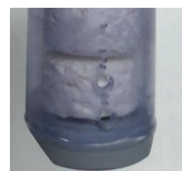
Figure 64: Holes in cylinder
