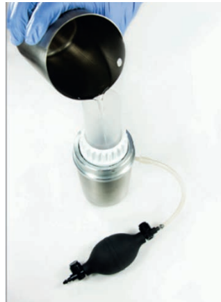
Figure 56: Membrane filtration funnel, DelAgua
