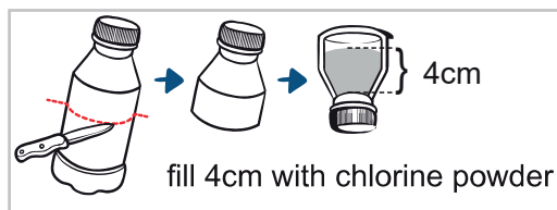
Figure 33: How to measure 100 g of chlorine powder with a 0.5L PET bottle
