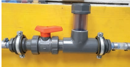
Figure 62: T-chlorinator in the laboratory at Eawag
